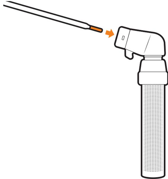
7. Twist electrode holder to tighten and securely grip electrode.
