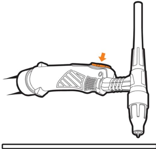
**14.** Touch the tip of the tungsten to the workpiece.
