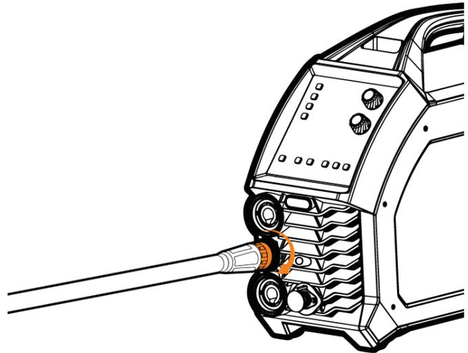
3. Now connect the polarity cable into the (-) dinse port, and twist it to lock it in place.
