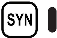
To activate Synergic mode, press the **Synergic Mode Button** while in MIG. You will see the Synergic Mode indicator light to the right of the button light up while Synergic Mode is active.
