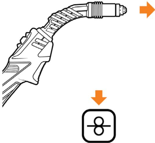
**18.** Feed extra wire out of the tip of the torch. Then slide the MIG tip along the wire back into place, screwing it in to secure it. Then slide the gas nozzle back into place. Cut the excess wire off just past the gas nozzle.
