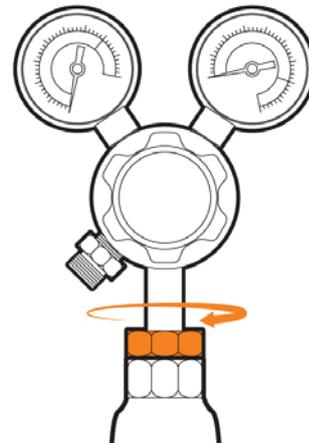
**22.** Screw in the supplied gas hose to the outlet port of the regulator.
