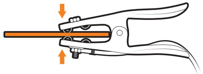
**9.** Strike electrode to the workpiece to initiate arc.
