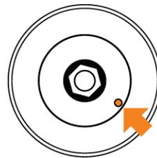
11. You can now lock the spool of wire in place by reinstalling the spool holder retainer nut (anti-clockwise to tighten).
