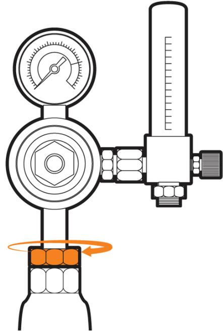
**7.** Connect gas hose to the flowmeter outlet using the twist nut to tighten the fitting securely.
