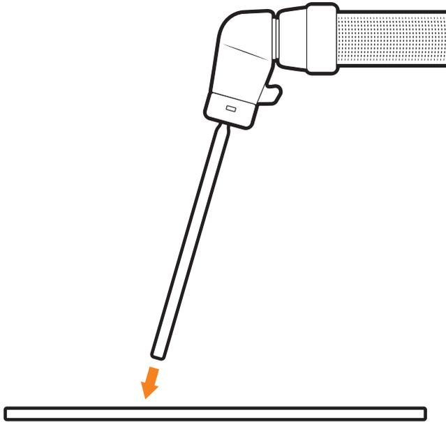
**10.** Drag along workpiece to weld. Pull the electrode away from the workpiece to finish weld.
