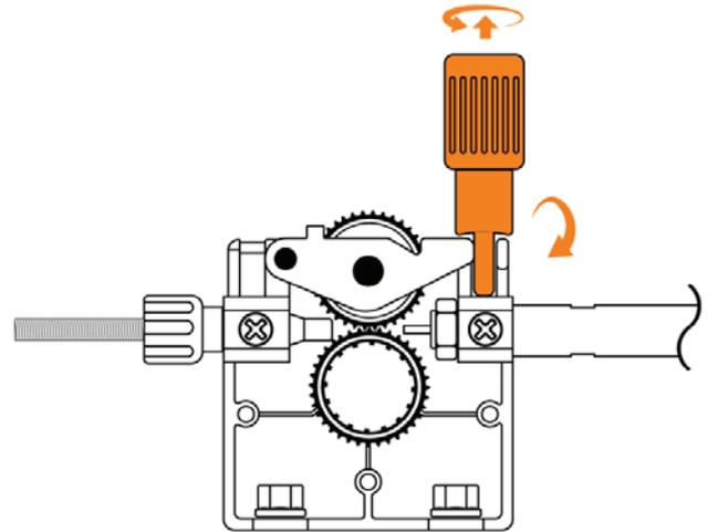
3. Lift the Upper Drive Roller Assembly up and out of the way. Then, loosen and remove the drive roller retaining nut by spinning it anti-clockwise.
